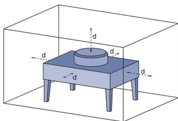
The sound pressure level represents the mean value on a parallelepiped surface that surrounds the model in free field with a perfectly reflecting surface, in compliance to EN 13487 standard.
